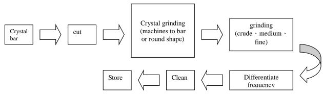
ii. Post-manufacturing process—quartz crystal (use silver, gold, nickel for electroplating, and the process would reduce crystal frequency. Fine tuning the electroplating that would reduce frequency error to 3~10ppm)
