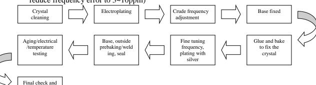
iii. Post manufacturing process—crystal oscillator (use silver, gold, nickel for electroplating, and the process would reduce crystal frequency.)
